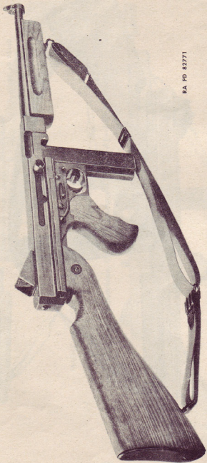
Figure 4 — Gun, Submachine, Cal. .45, Thompson, M1 and M1A1 — Right Side View
