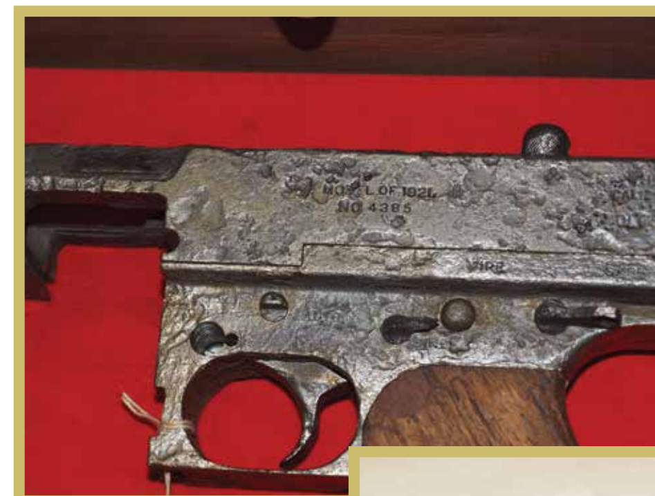
A well traveled S/N 4385 after storage in water. Note how clean the interior is compared to the outside.
