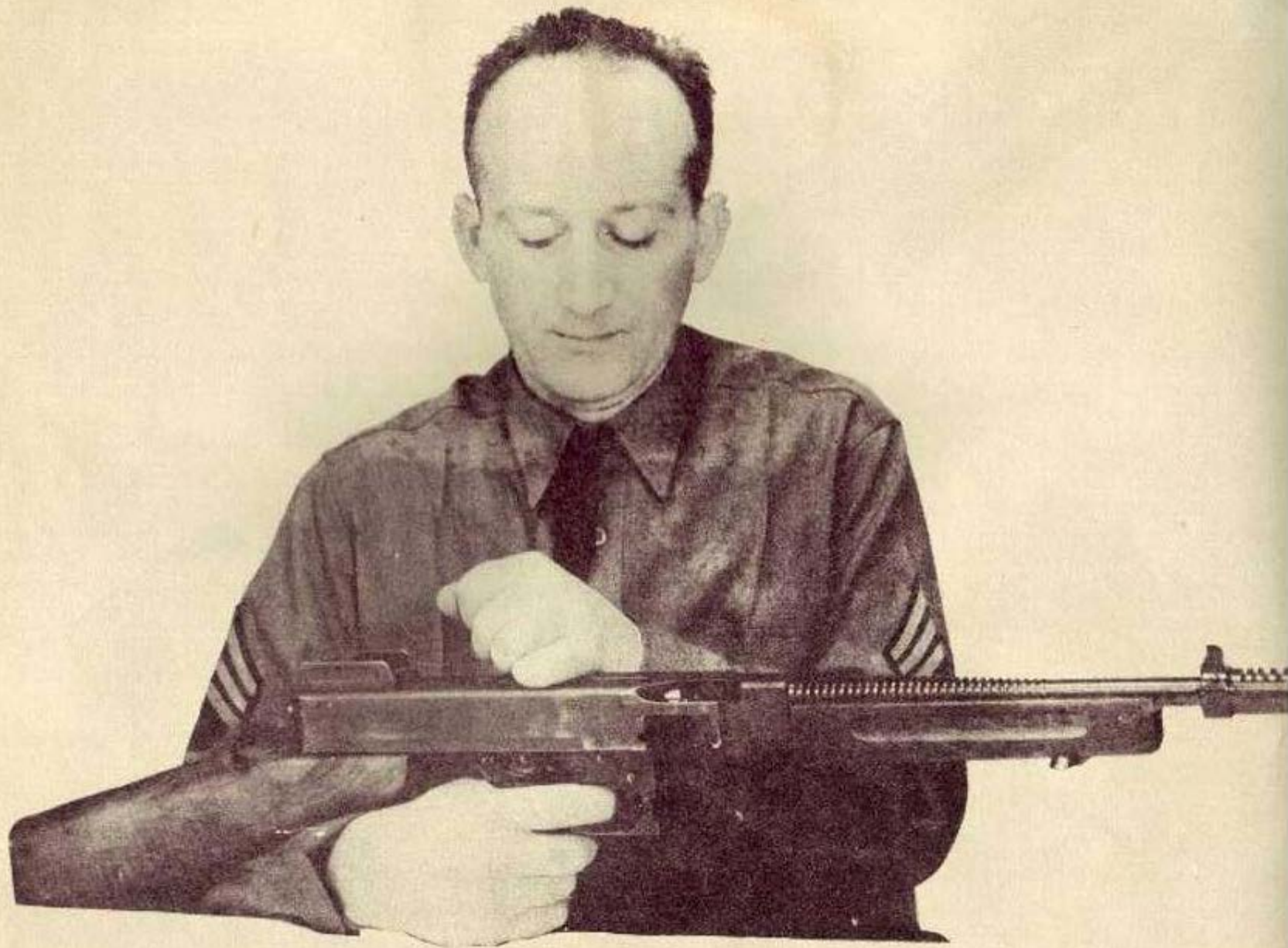
Fig. (2): Pull TRIGGER and allow recoiling parts to move forward slowly. This is done by retarding the forward movement of the ACTUATOR KNOB. ( Note : the BOLT must never be allowed to go forward on an empty CHAMBER.)
