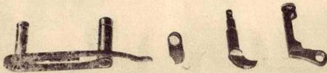
Fig. (20): Replace TRIGGER, TRIP, SEAR AND SEAR LEVER with their contained springs in their correct positions in the FRAME. ( Note : Be sure that forward end of SEAR LEVER rests on DISCONNECTOR.)
