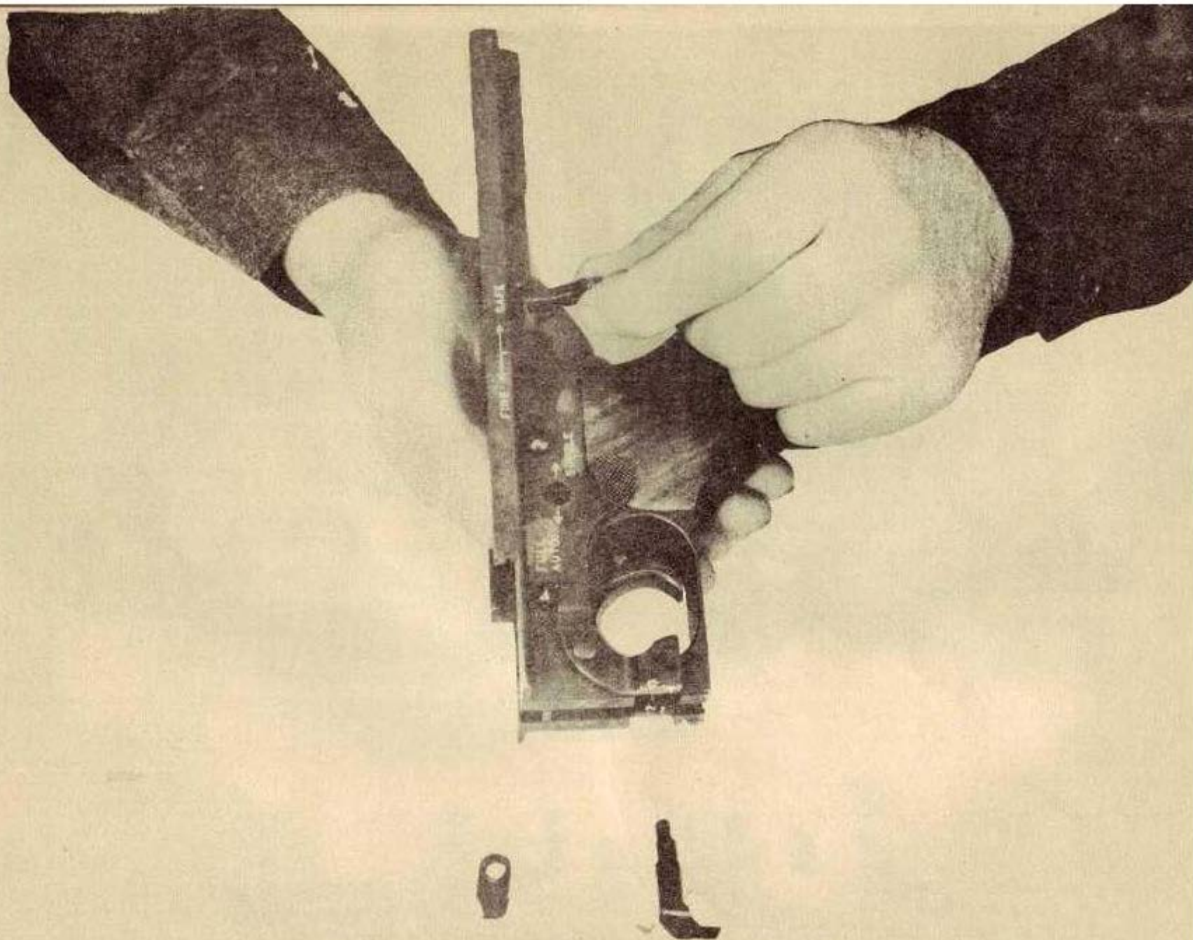
Fig. (22): Insert SAFETY LEVER and secure with long finger of PIVOT PLATE. ( Note : This is done in the same manner that the lever was removed; by levering the finger down with a tool.)
