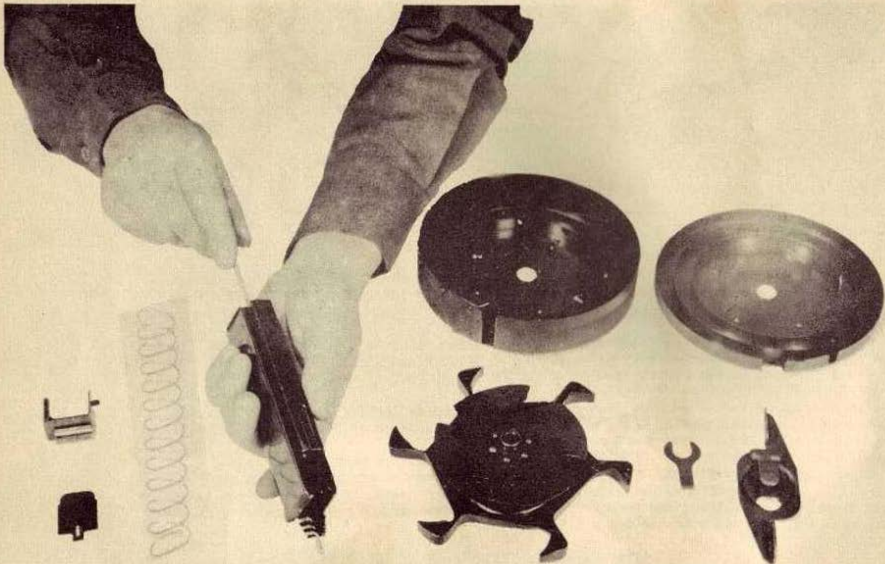
Fig. (6): It is imperative that magazines be given the best of care and kept in perfect condition. They should be disassembled, wiped clean and dry, and thinly coated with oil. Dirt that gets into them through careless handling must be removed. Care must be exercised to avoid denting or bending, especially the lips of the mouth of the BOX MAGAZINE (XX).
