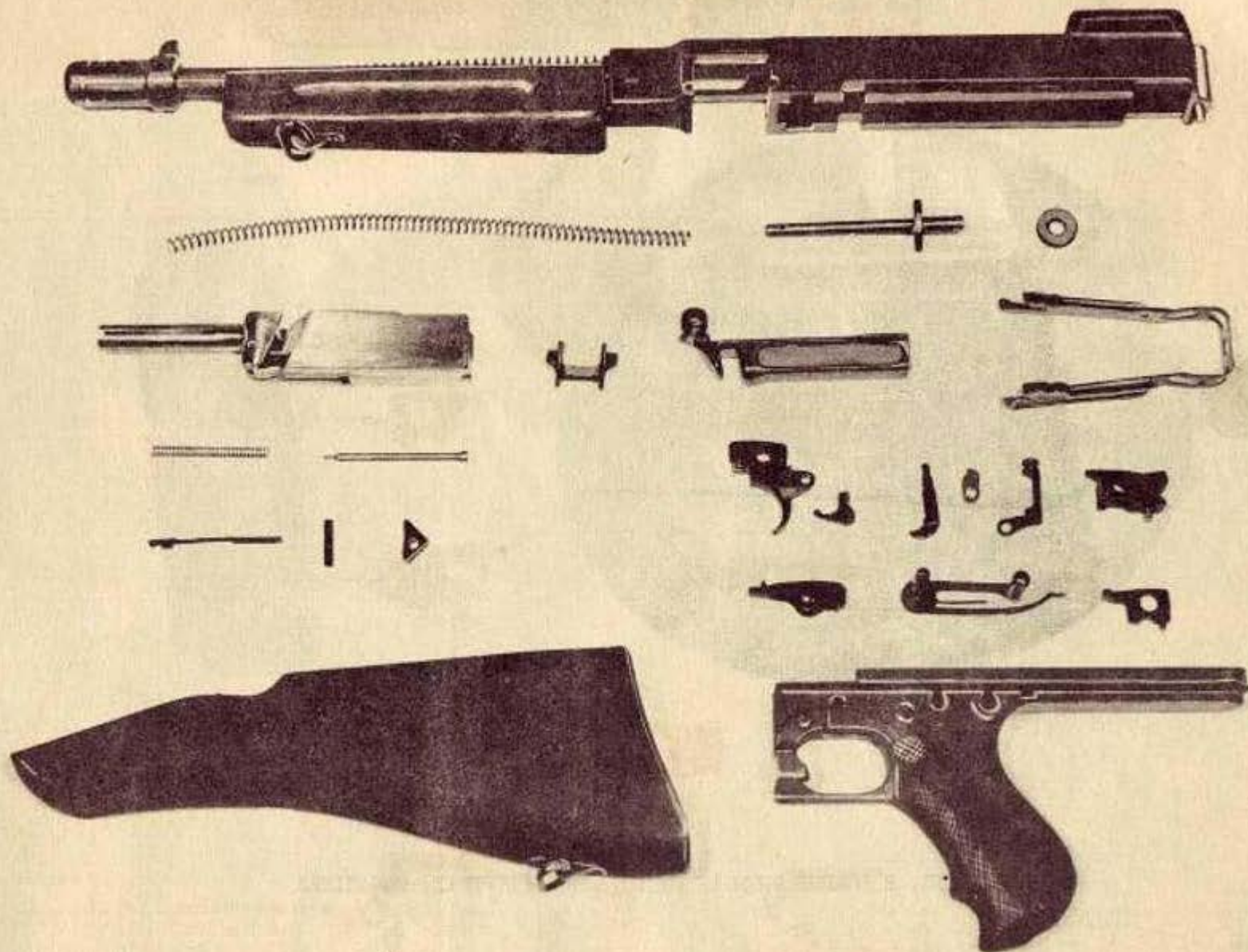
FIG. 7 COMPLETE DISASSEMBLY OF GUN FOR CLEANING (NOT INCLUDING FORE-GRIP)
