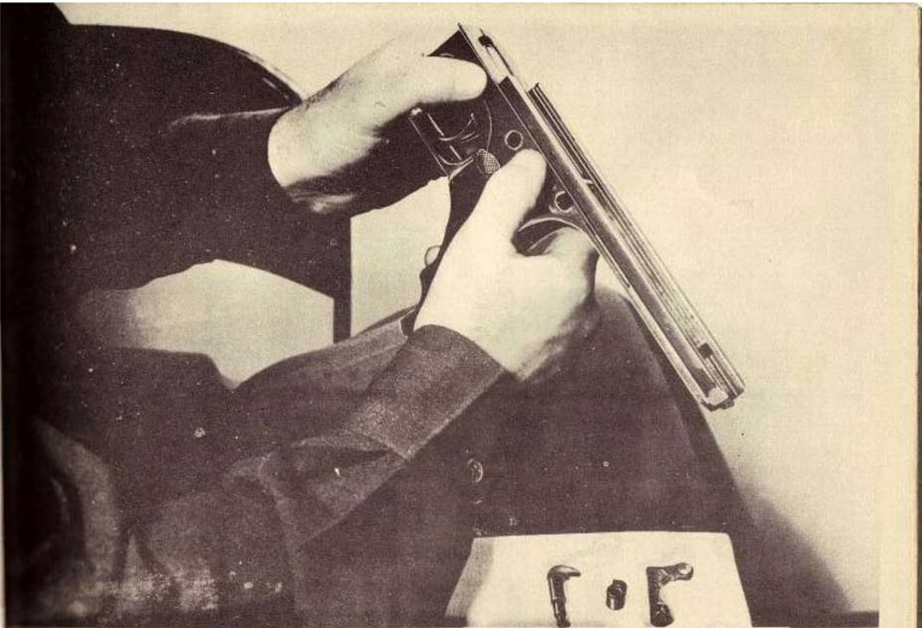
Fig.(17): Holding the FRAME in both hands, apply pressure with the balls of the thumbs to the TRIGGER and SEAR PIVOTS. Press evenly on both pins until the PIVOT PLATE protrudes on the other side far enough to permit withdrawal.
