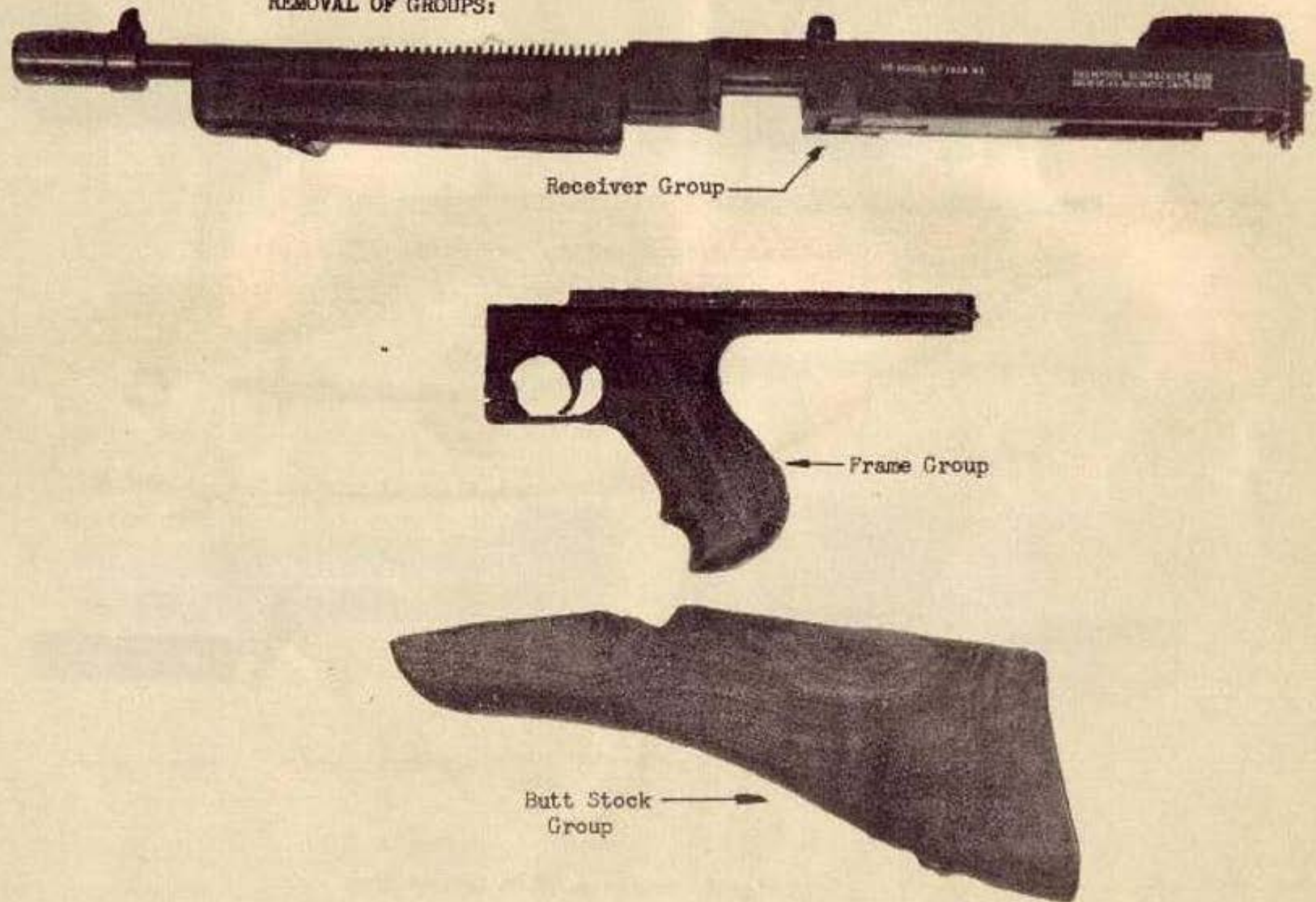
Fig. (3). Three component groups of the gun
