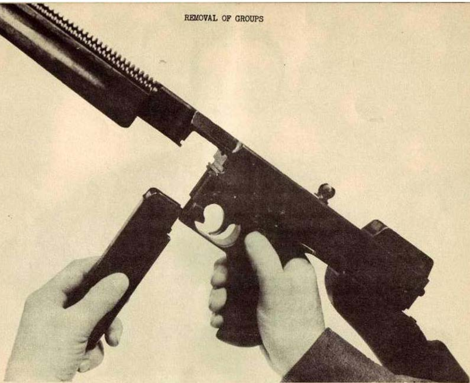
Fig. (1): Hold the gun in the right hand by the REAR GRIP and raise up on MAGAZINE CATCH. Slide MAGAZINE from MAGAZINE GUIDEWAYS. (Either BOX or DRUM MAGAZINES).
