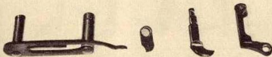
Fig. (19): Turn FRAME upside down and empty contained parts into the palm of the other hand.
