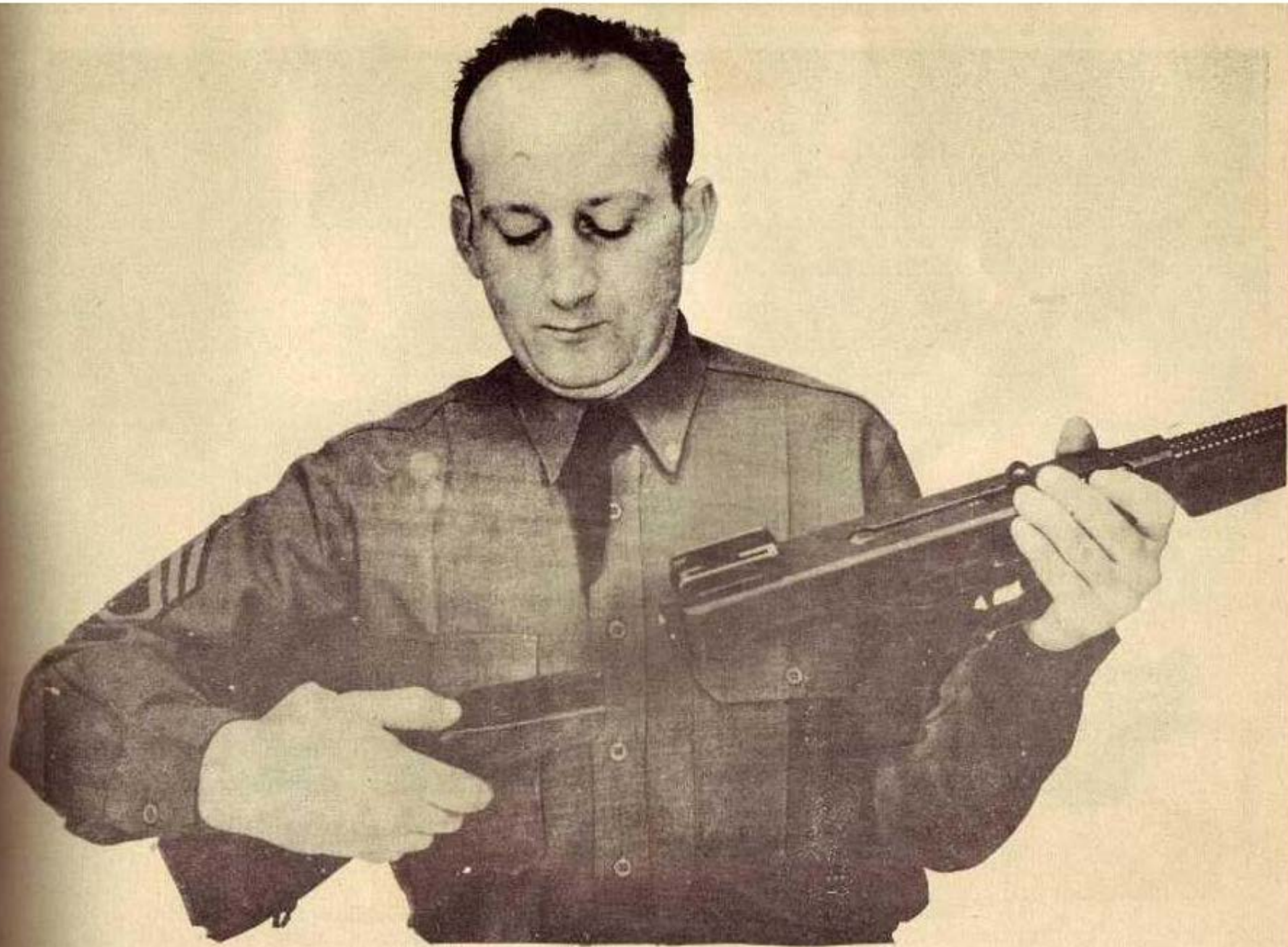
Fig. (3): Remove BUTT-STOCK by pressing down on BUTT-STOCK CATCH BUTTON and sliding BUTT-STOCK from the BUTT-STOCK GUIDEWAYS on the FRAME.
